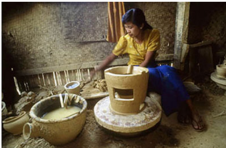
Figure 13. A ceramic cook stove saves fuel in Myanmar
