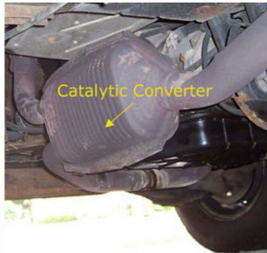
Figure 21. Catalytic converter mounted in a car's exhaust system
