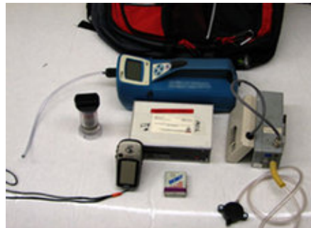
Figure 6. Backpack system for measuring exposure to fine particulate air pollution
